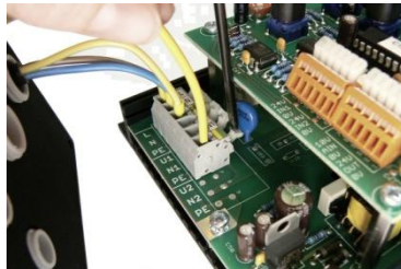
Fig. 8 - connecting conductors to terminals
