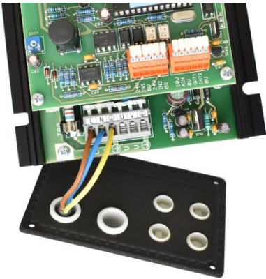
Fig. 5 – disassembly of the part with outlets
