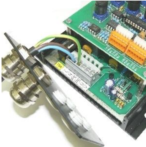
Fig. 6 - Removal of the part with outlets
