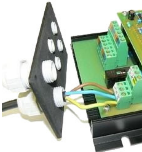
Fig. 6 - Removal of the part with outlets
